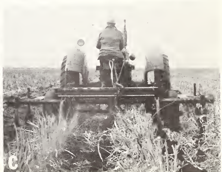
FIGURE 3.— A , Side, and B , front view of stubble-mulch plows constructed at the experiment station in 1945. Note the heavily reinforced construction of frame. C , Plow operating in sorghum stubble.
